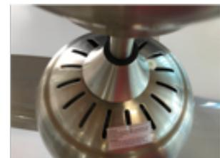
3/ Put the two cups on the down rod correctly, remove the bolt-pin kit from the motor and the screws, pass the wires inside the down rod and position the down rod correctly on the motor (only 1 possible direction, hanger ball to the ceiling). Replace the bolt-pin kit, by taking care to not damage the wires running inside, then tighten strongly. Retighten the screws on the down rod so that it is firm.
