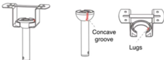
**Be careful to not damage the electrical wires and not wedge them between the hanger ball and hanger bracket. Make sure that the ceiling fan is securely locked. Concave groove of hanger ball must be putted into the bracket lugs.**
